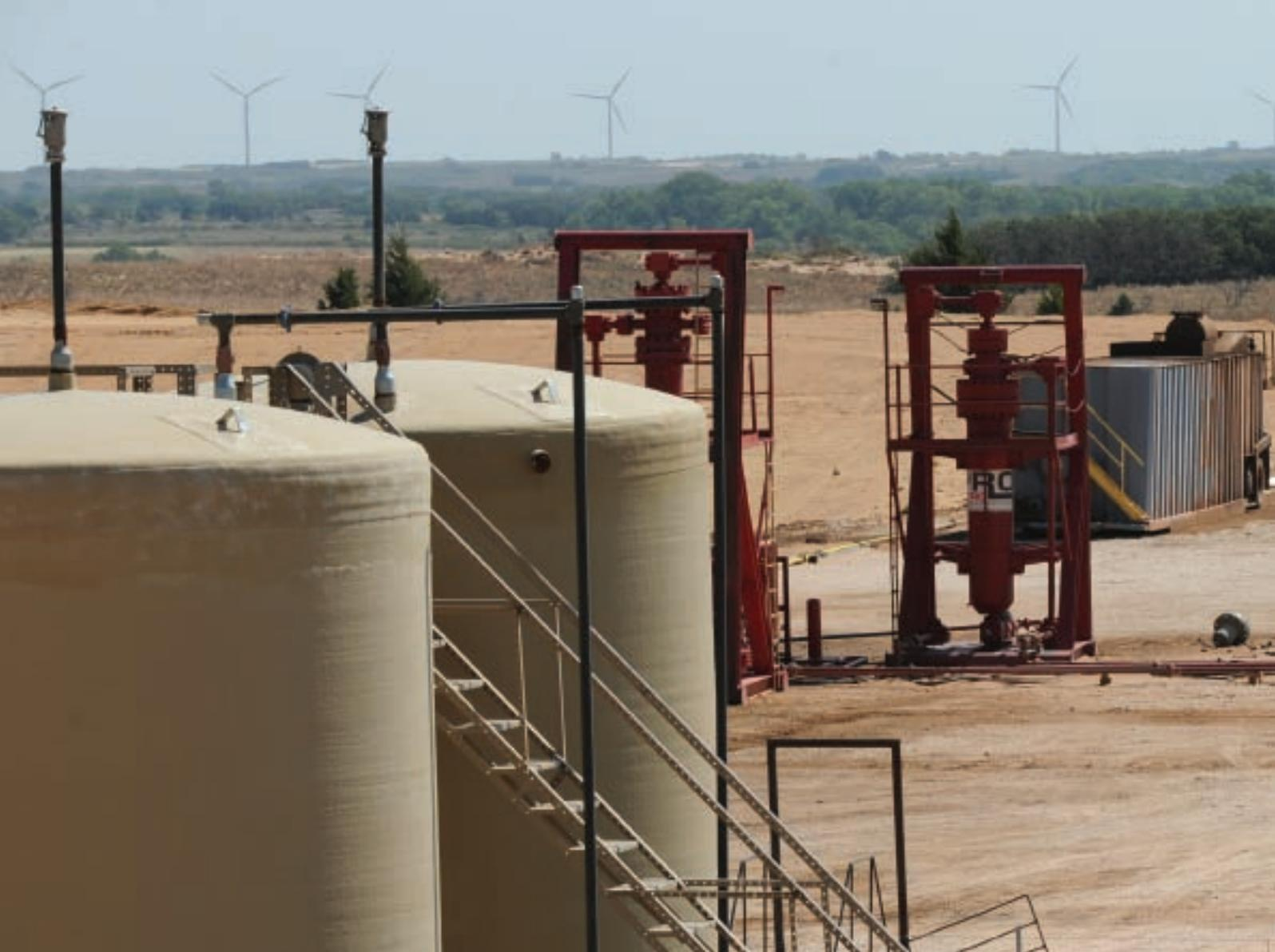
**Cordillera's A.C. Smith 41-2HB in Wheeler County, Texas, had first-24-hour production of 17 million cubic feet of gas, 1,554 barrels of gas liquids and 632 barrels of oil from the Britt bench of the Granite Wash conglomerate in the midst of one of several Texas Panhandle wind farms.**
